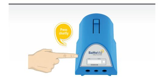
The light bars first rise to 100 % and then fall back to the actual battery capacity. One light bar corresponds to a battery capacity of 10 %.
