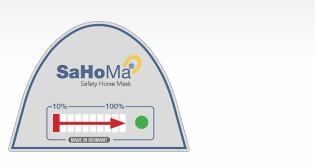
When the set time has elapsed, the aerosol production stops. The SaHoMa®-II control unit indicates the end of the inhalation process by two light bars running synchronously from the center to the right and left.
