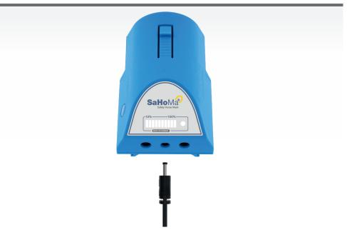
The charging process of the lithium polymer battery starts. As long as the lithium polymer battery of the SaHoMa®-II control unit is charged, the multifunctional light flashes green.
