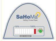
The display shows a light bar, which is on the **right** and the multifunctional light flashes **alternately red and green.**
