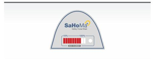
This display appears for approx. 2 seconds and then disappears again. The display shown above shows 8 light bars, which corresponds to a battery capacity of 80%.
